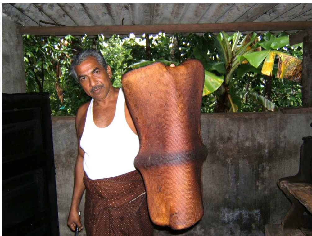
Figure 32. Natural rubber (polyisoprene) after chemical, mechanical, and thermal treatments, as a finished commercial product
